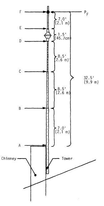
fig. A1. Tower/antenna configuration.
